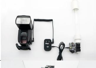
Connect the valve to the Aux port of your Pluto Trigger using the valve cable. Connect your flash to the camera port of the Pluto Trigger. Point the IR emitter on the Pluto Trigger to your camera.
