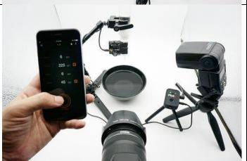
Turn on your Pluto Trigger. Launch the Pluto Trigger app on your phone. Set the IR settings to match your camera model. Select <u>Droplet</u> mode from the menu. Press the start button to test. The Pluto Trigger should send IR commands to trigger your camera, release two droplets and then trigger your flash.
